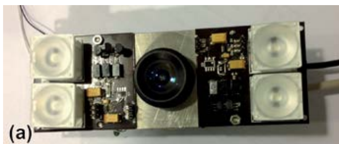
(a) 3D camera prototype, (b) intensity image, (c) range image.
